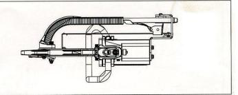
Note: New design of pusher (with two ears), you can load C-Ring first then pull pusher later. It is easier loading C-Ring.
